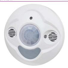
SB-CMS-12in1 12 in 1 sensor includes temperature sensor, PIR motion sensor, LUX sensor ,ultrasonic sensor, dry contacts, IR received, IR emitter, 2channel 5A relay output and logic block. The logic block can combine all sensors for different applications. It supports HDL security mode and command.
